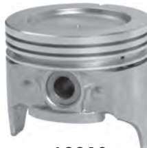
L2213 OLDS 425 C.I. 1965-1967 9:1 Compression Bore 4.125-4.185 Ring Set-up 2) 5/64, 1) 3/16
