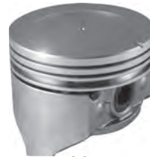
L2214 OLDS 425 C.I. 1965-1967 10:25 to 1 Compression Bore 4.125-4.185 Ring Set-up 2) 5/64, 1) 3/16
