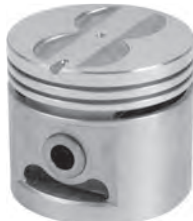
L2153 OLDS 215 C.I. 1961-1963 4 Valve Reliefs Bore 3.5000-3.560 Ring Set-up 2) 5/64, 1) 3/16
