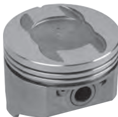
L2257 PONTIAC 428 C.I. 1967-1969 Bore 4.1200- 4.180 Ring Set-up 2) 5/64, 1) 3/16
