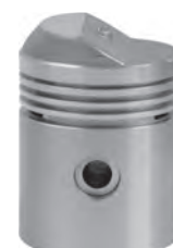
L944 GMC 228 C.I. Wedge Dome Bore 3.5626-3.6626 Ring Set-up 1) 3/32, 2) 1/8, 1) 3/16
