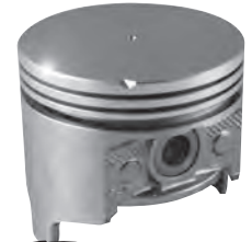
NEW!! L2320 OLDS 350 V-8 FLAT TOP 10.5:1 RATIO Bore: 4.057-4.117 Ring Set-up: 2) 5/64, 1) 3/16
