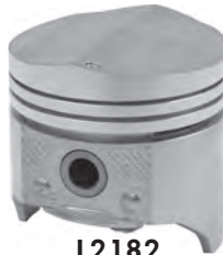
L2182 LINCOLN Late 430 1963-1965 Bore 4.300-4.360 Ring Set-up 1) 5/64; 1) 3/32; 1) 3/16
