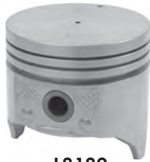
L2120 LINCOLN Early 430 1959-1962 Bore 4.300-4.360 Ring Set-up 1) 5/64, 1) 3/32, 1) 3/16
