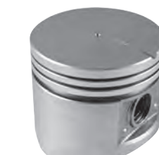
L2018 FORD 312 Y-BLOCK Bore: 3.800-3.880 Ring Set-up: 1) 5/64, 1) 3/32, 1) 3/16
