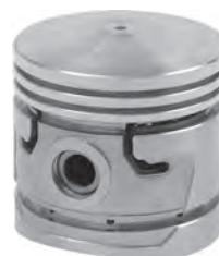
E135 FORD 1939-1953 V-8 Flathead Bore 3.1875-3.3125 Ring Set-up 2) 3/32, 2) 3/16
