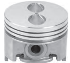
L2269 PONTIAC 389 C.I. 1959-66 Bore 4.0625-4.1225 Ring Set-up 2) 5/64, 1) 3/16
