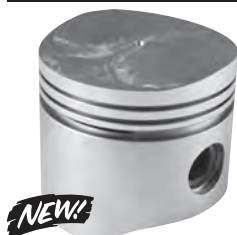
L2222 DODGE/PLYMOUTH 273 V-8 10.25 TO 1 RATIO Bore: 3.625-3.685 Ring Set-up: 2) 5/64, 1) 3/16
