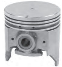
L2133 OLDS 324 C.I. 1954-1956 V-8 Bore 3.875-3.935 Ring Set-up 2) 5/64; 1) 3/16
