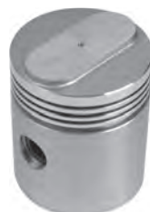
L986 GMC 228 C.I. Flat Dome Bore 3.5626-3.6425 Ring Set-up 3) 3/32, 1) 3/16
