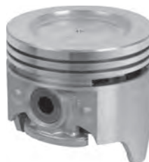
EP2416 STUDEBAKER 289 C.I. 1956-1964 Bore 3.5625- 3.6225 Ring Set-up 2) 5/64, 1) 3/16
