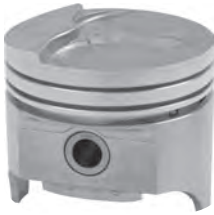
E969 LINCOLN 462 1966-68 V-8 Bore 4.380-4.440 Ring Set-up 1) 5/64; 1) 3/32; 1) 3/16
