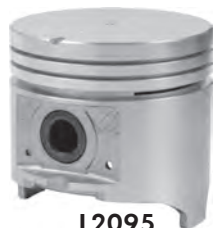
L2095 CHRYSLER/DODGE 413 C.I. 1959-64 Bore 4.1875-4.2475 Ring Set-up 2) 5/64, 1) 3/16
