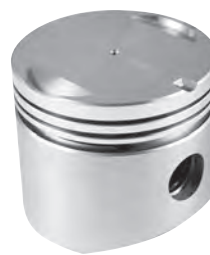
L1087 DESOTO 330 V-8 1956 Bore: 3.718-3.778 Ring Set-up: 2) 5/64, 1) 3/16
