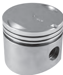
L1037 DESOTO 291 V-8 1955 Bore: 3.718-3.778 Ring Set-up: 2) 5/64, 1) 3/16
