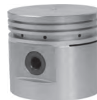
L2027 STUDEBAKER 259 C.I. 1959-1964 Bore 3.5625-3.6225 Ring Set-up 2) 5/64, 1) 3/16
