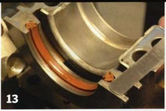
Here I are checking the amount the ends of the seal protrude from the cap with the seal pressed in place. You need 0.010-0.020 inch sticking out at each end so the seal will crush 0.020-0.040 to hold it tightly in the groove to keep it from spinning with the crank. This is very important.
