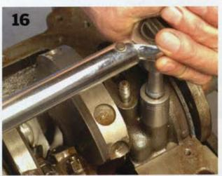
> Some people spread a very thin coat of sealer on the flat cap surfaces, but I don't think it's necessary. Do not apply any sort of sealer to the ends (where they butt) of either a rope or lip seal, however. Then install the cap and torque to spec.
