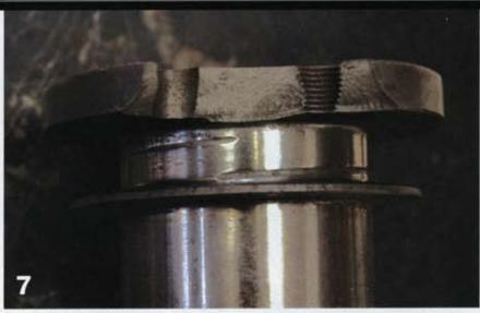
> The Ford flathead V-8 has this deep, spiral groove to direct oil back to the pan, so a lip seal obviously wouldn't work (nor are any available).
