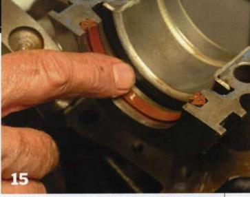
If the engine will sit before it's started, spread a thin coat of oil or grease on either a new lip or rope seal so it isn't dry at initial startup.
