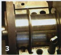
> These engines came only with rope seals, but fortunately the crank flange was not knurled and the groove is even and symmetrical. Better, the raised, thin flange between the seal and the bearing, while not exactly an oil slinger, is still a very good oil shield, diverting oil back into the pan through a hole in the bottom of the cap. Given the chunk of seal that was missing, this was working pretty well, GM didn't want their Caddys dripping oil.
