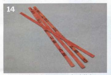
If the seal doesn't protrude the proper amount from the block or cap, you can get from Best these special shims made from composition gasket material to adjust it. Do not try brass shim stock or filling the groove with silicone to shim the lip seal. I can tell you from experience it doesn't work.
