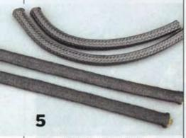
Just so you know, the "bad" new asbestos-free rear-main seals look like the examples at the bottom. They are black and tightly woven. Older seals with asbestos are more loosely woven and lighter in color. The Best Gaskets with GraphTite at top look like dreadlocks and are silverygray in color.
