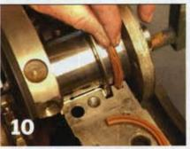
Next, you can simply slide the lip into the groove in the block, as shown. You can't do this with a new rope seal when the crank is in place like this. It can be done with a "Sneaky Pete" tool, but it's not a pretty process.
