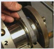
If you were rebuilding the engine, you'd have the crank journals polished, including the seal surface. Since this one was neither scored nor scratched, I tore a piece of medium emery cloth to the right width and used it to lightly polish the journal. Use an air gun to blow any grit or debris out of the channel afterward.
